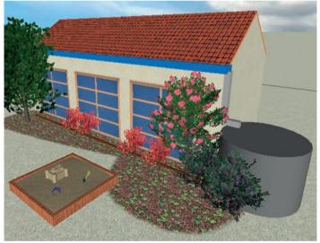
Fig. 20 A simple rainwater harvesting system (Tsirogiannis, 2010)
